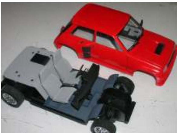
The interior builds up off the floor. It is a basic interior, two seats, dashboard and shifter. I painted the floor Tamiya German Gray. The seat and deck were sprayed with Scale Motorsport Faux Fabric grey, to represent a cloth material finish.
