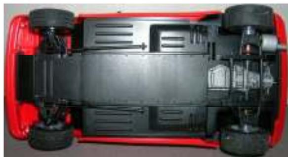
This kit is a curbside, the only engine detail is molded onto the bottom of the chassis. A muffler is the only additional piece. Since there is not much there I did not bother to paint the chassis (it is molded in black) but I did paint the engine metallic gray. The front suspension is steerable, with spindles and tie rod while the rear is a metal axle.
