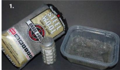
Start with a fine grade of steel wool. In this case I used #0000. Pick a container that you can throw away when the process is completed, as there is quite a bit of rusty residue in the container when the process is finished. Put a number of small amounts of steel wool in the container, and add water so that the steel wool is submerged in it. Lastly, add salt as this speeds up the process of turning the steel wool into rust.
