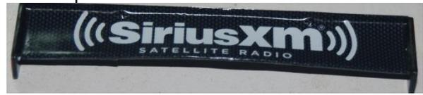
The rear wing is a three piece assembly, the red end plates are decals and the wing was painted
