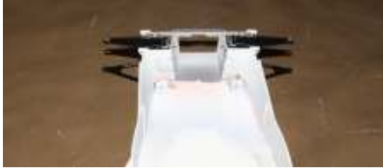
Photo 4. Front suspension mounted to lower half of tub. It was necessary to modify the top and bottom pieces of the tub to accept the aftermarket suspension and bulkhead components.
