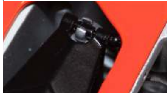
Photo 10. Stiff wire with the insulation removed and 2 modified resin oil fittings used to make the front endlinks.
