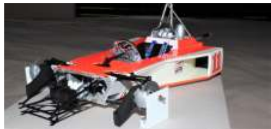
Photo 11. Short nose bracket installed. Brace was added to center of the bracket and battery tray both built from sheet plastic. The battery tie-
