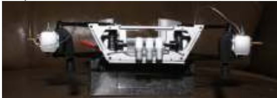
Photo 5. Front uprights and brake assemblies installed. Fluid lines are beginning to be installed but will not be completed until the top of the tub is added.
