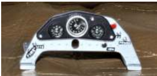
Photo 6. Labels being added to dash assembly. Labels were made using Microscale black stripes and white lettering.
