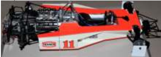
Photo 14. Chassis waiting for final details. Back of dash has wires running to engine. Tub extensions added.
