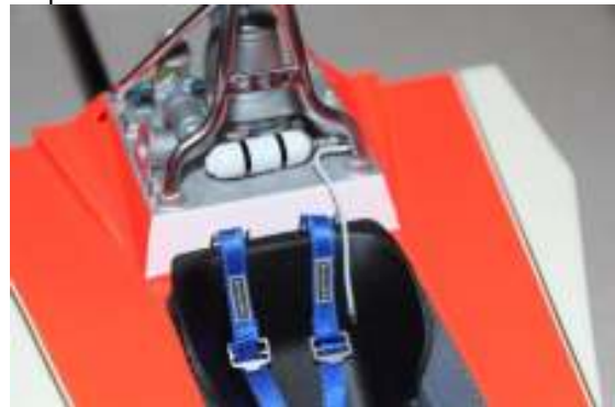
Photo 9. A short piece of stiff wire with white insulation and a modified resin oil fitting used to make the oxygen supply tube. Top half of Swirl Pot made from the stem of a plastic champagne glass found at the 99 Cent Store.
