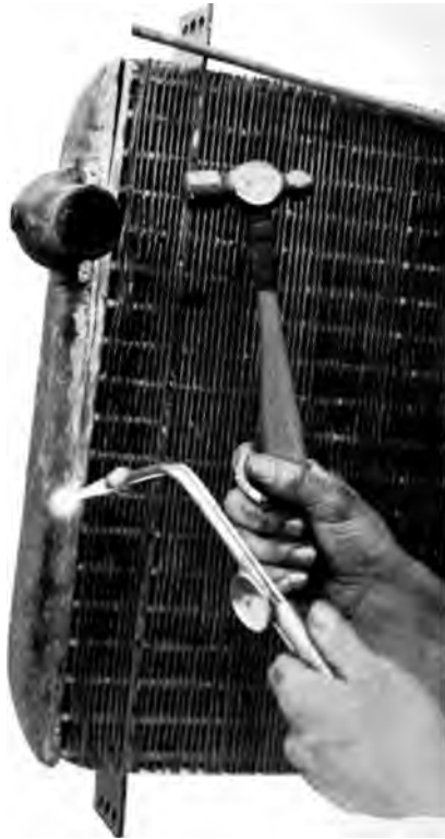
Fig. 83 Removing the Bottom Tank
