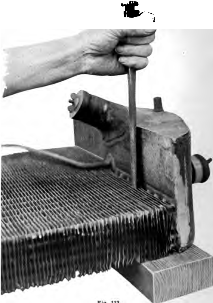
Fig. 112 Cutting Tank From Damaged Core
