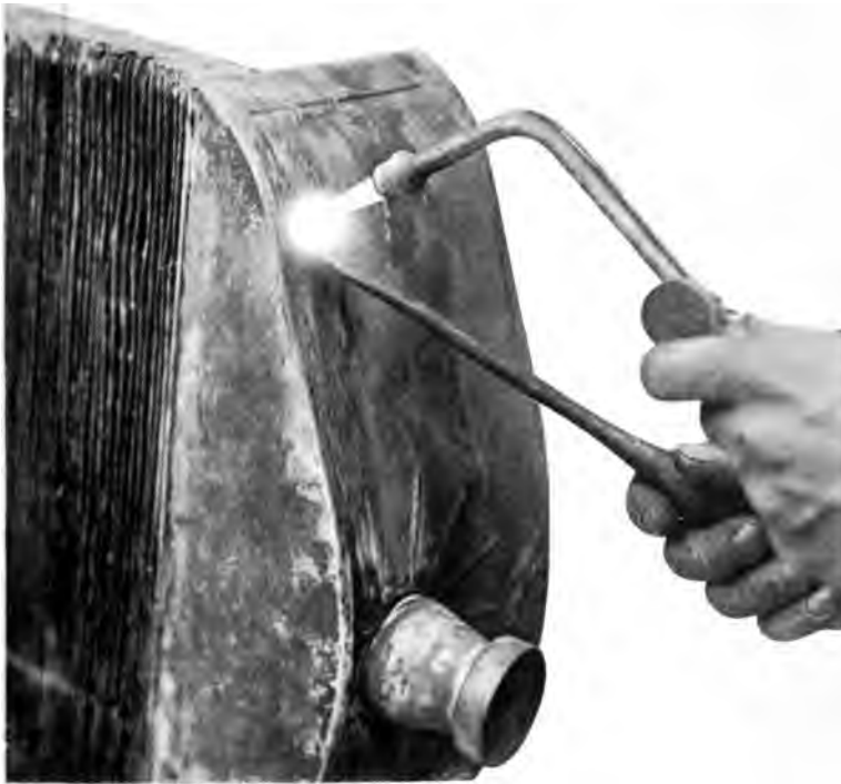
Fig. 85 Removing the Front Wall
