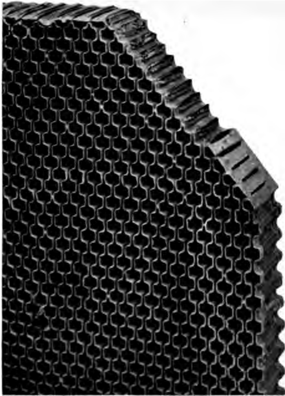
Fig. 117 Heading a Diagonally Cut Core
