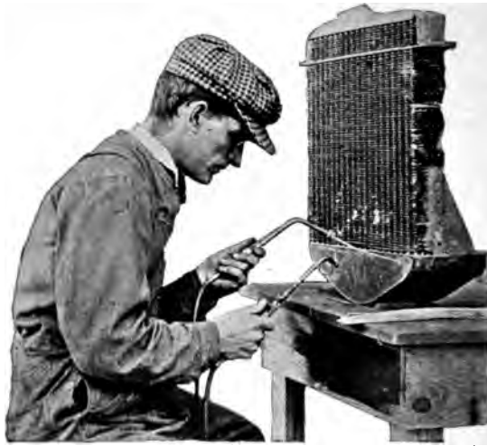
Fig. 78 Resoldering Tubes in Top Header
