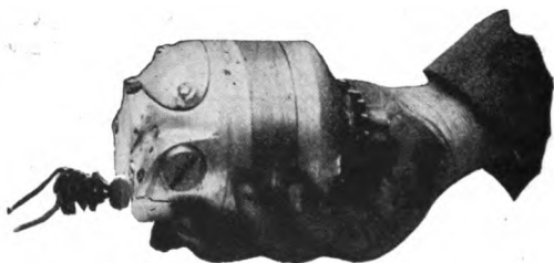
"REX" LIGHTING GENERATOR WITH CUT-OUT AND REGULATOR IN SAME CASE.
