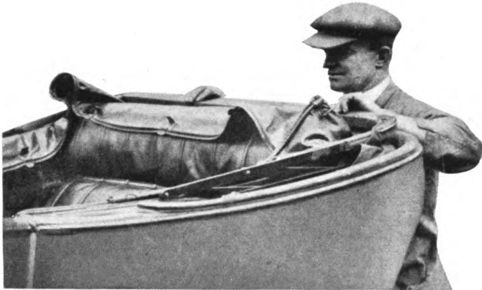
TOP CONTAINER BUILT INTO THE BODY This English device preserves the graceful lines of the body when the top is down, the top being entirely concealed from view.
