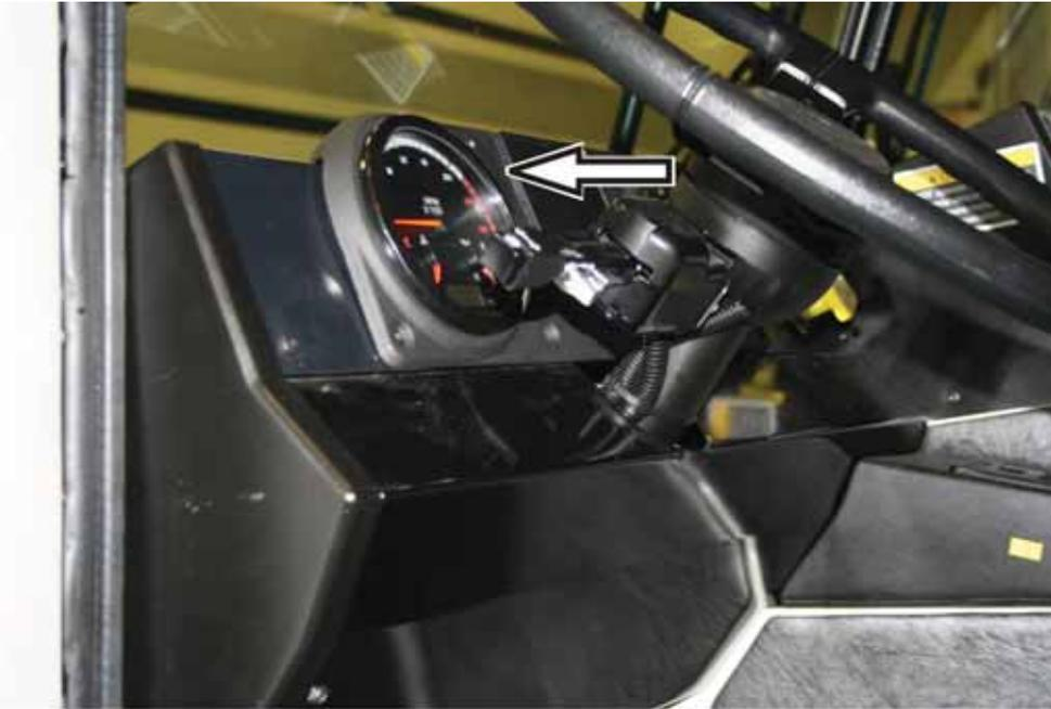
d. Remove the long access panel located above the mirror switch.
