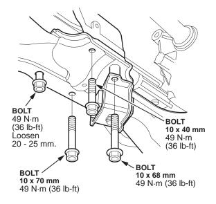
11. Using a transmission jack, carefully lift the engine until the rear engine bracket lifts off the rear part of the subframe.
