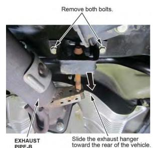
10. Remove three of the rear engine mount bracket bolts from the subframe. Loosen the fourth bolt 20-25 mm and make sure that it is still threaded.
