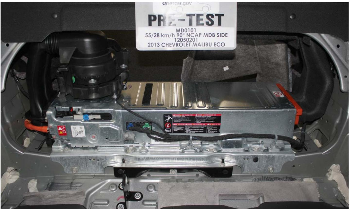
No. 019 Pre-Impact View of Propulsion Battery Venting System(s)
