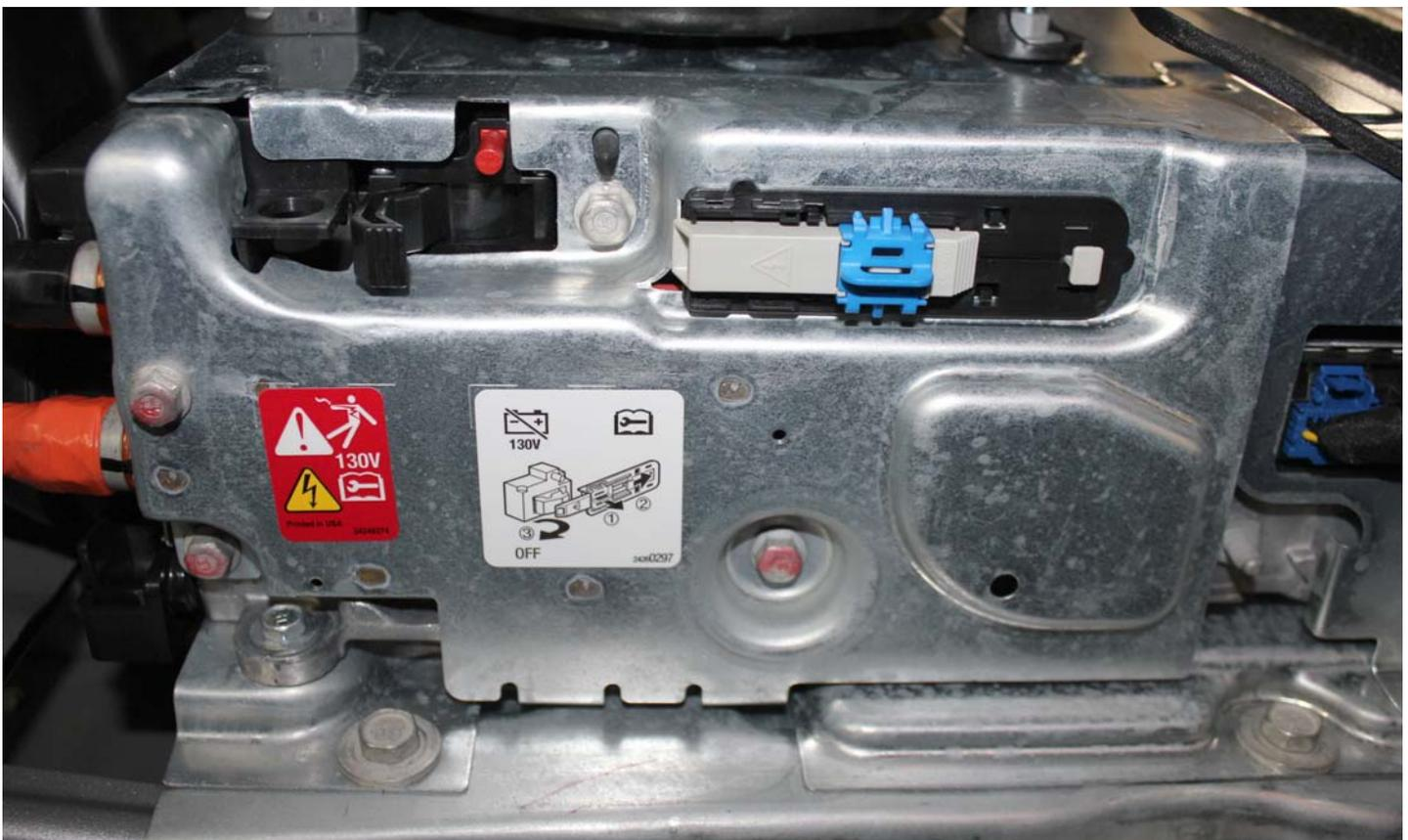
No. 007 Manual High Voltage Service Disconnect Removed
