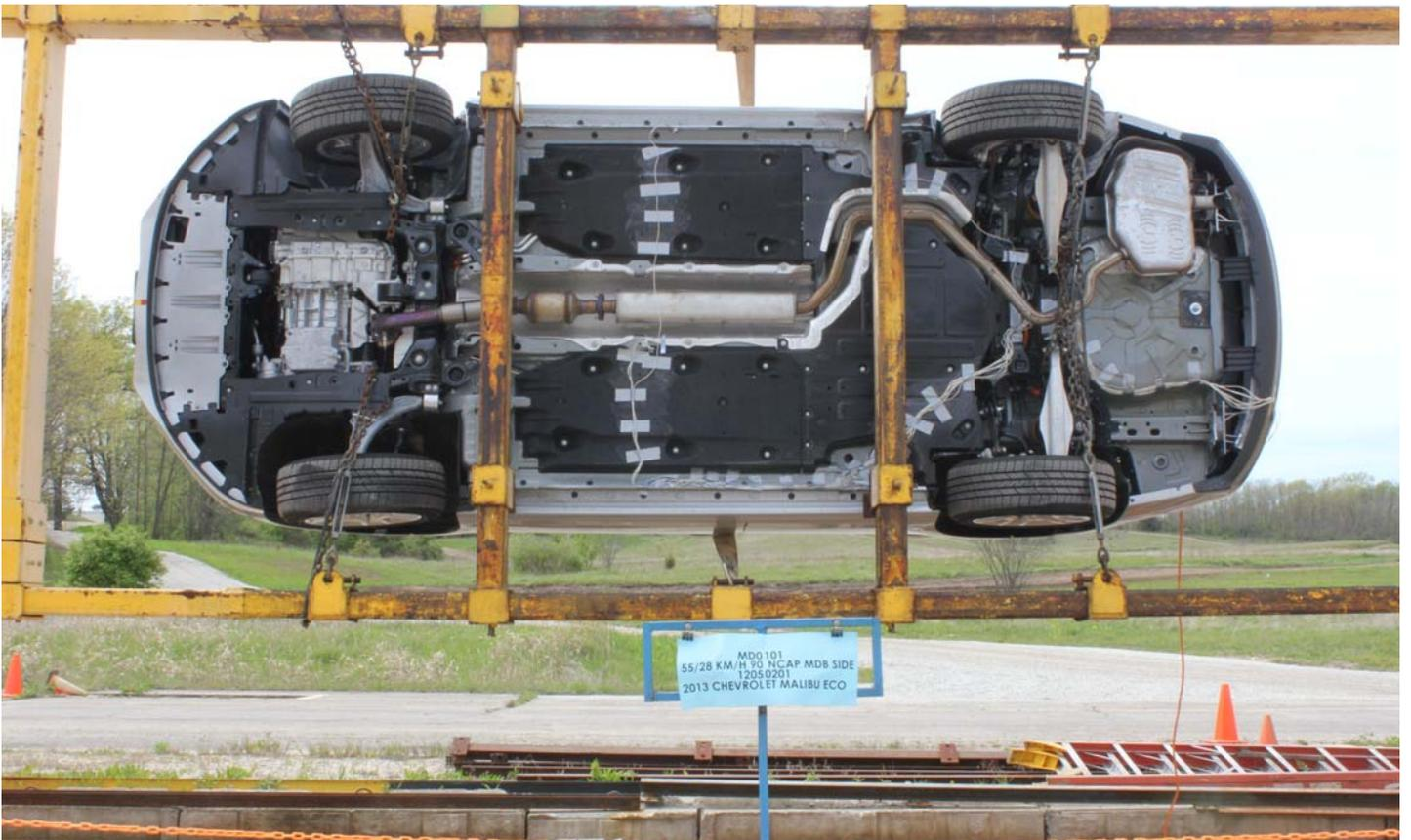
No. 028 FMVSS No. 305 Static Rollover at 90°
