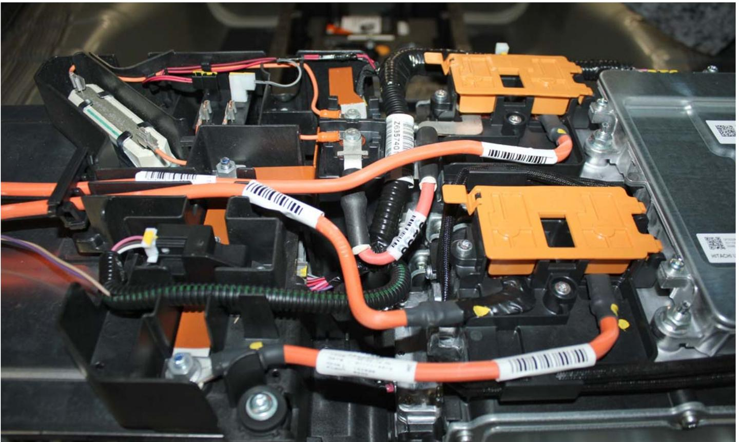
No. 014 Pre-Impact View of Propulsion Battery Module(s)
