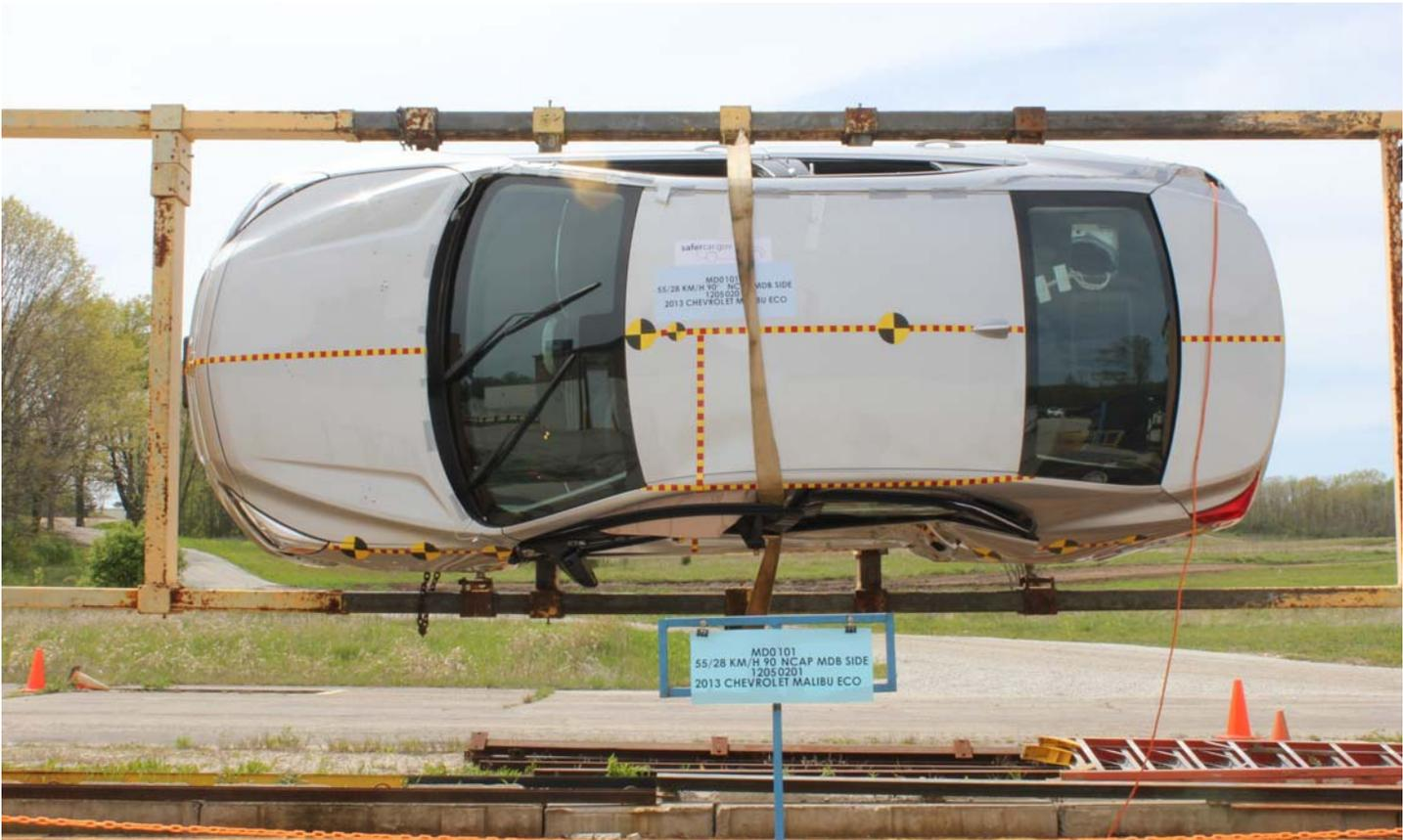
No. 030 FMVSS No. 305 Static Rollover at 270°
