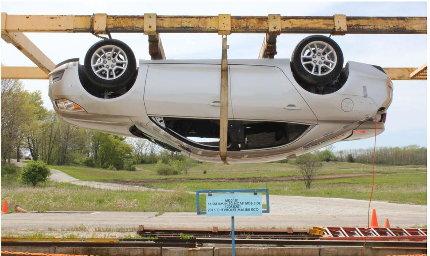
No. 029 FMVSS No. 305 Static Rollover at 180°
