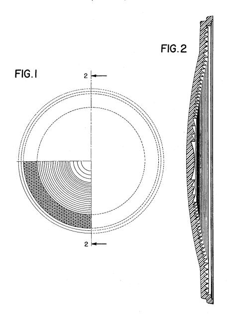
Fig. 1 is an elevational view of a reflex lens embodying my invention; and
