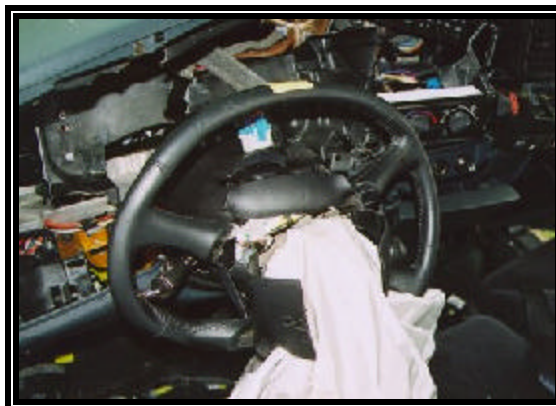
Figure 8: View of the deformed steering wheel.
