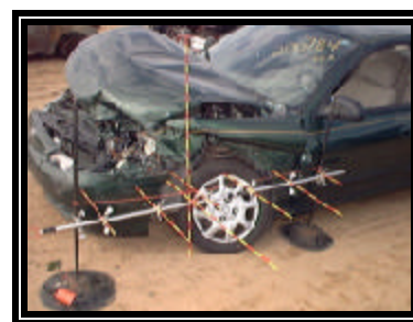
Figure 4. Left front side damage to the Elantra
