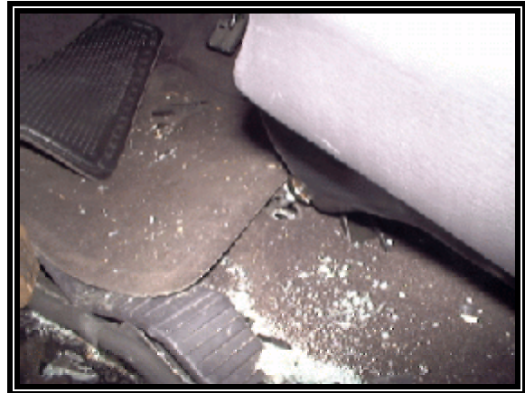
Figure 7: Buckled floor pan and left front seat anchor.
