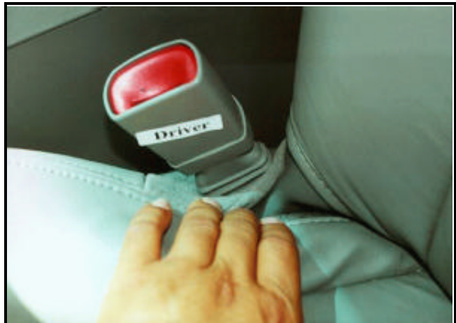
Figure 7. Driver's seat belt pretensioner—in fired position
