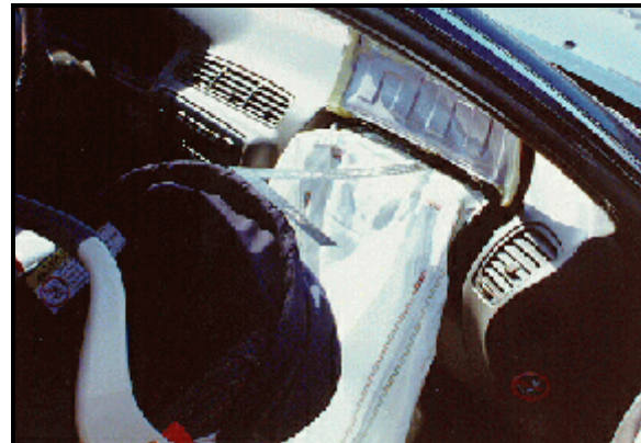
Figure 12: Case vehicle's front right seating area showing distance [23 cm (9 in)] from back of Rear Facing Child Safety Seat to front right passenger's air bag module (case photo #24)
