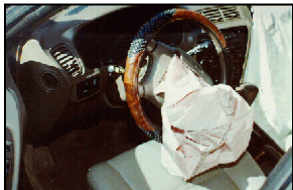
Figure 7: Case vehicle's driver seating area showing deployed driver air bag; Note: driver's seat is near its forward-most position (case photo #17)
