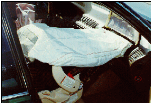
Figure 9: Case vehicle's front right seating area showing deployed, untethered, front right passenger air bag extended over Rear Facing Child Safety Seat (case photo #23)
