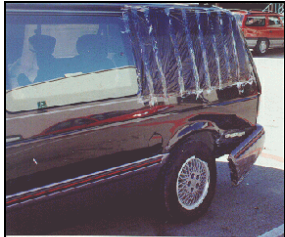
Figure 6: Damage to other vehicle's left quarter panel from impact with case vehicle; Note: left back glazing was shattered (case photo #45)
