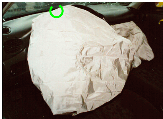
Figure 10: Case vehicle's deployed driver air bag showing no apparent skin evidence; Note: small cut (circled) found near seam (case photo #33)
