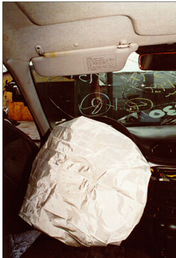
Figure 9: Case vehicle's driver seating area showing left "A"-pillar, windshield, front header/sun visor, and front surface of deployed driver air bag with no apparent evidence of occupant contact; Note: faint grease smears and black scuffs are present on air bag that occurred during deployment from contact with underside of cover flaps (case photo #31)
