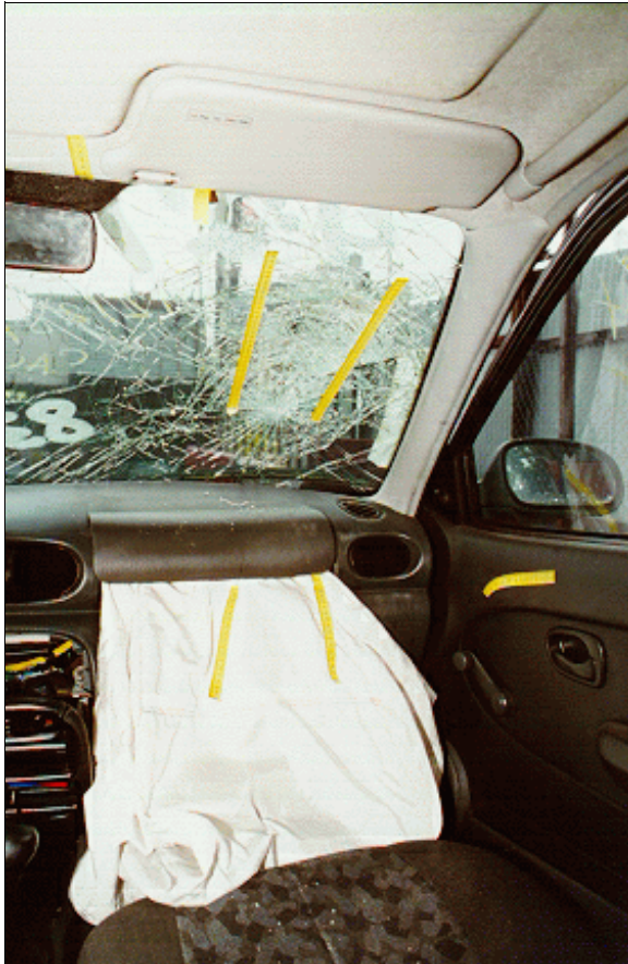
Figure 5 Vertical view of case vehicle's front right passenger seating area with tape highlighting apparent occupant contacts (case photo #34)
