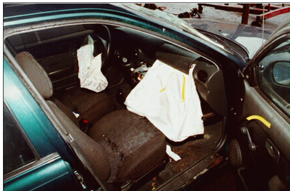
Figure 8: Case vehicle's front right seating area and interior of front right door showing seat position and evidence of occupant contact on air bag and scuff on door's interior surface (case photo #27)
