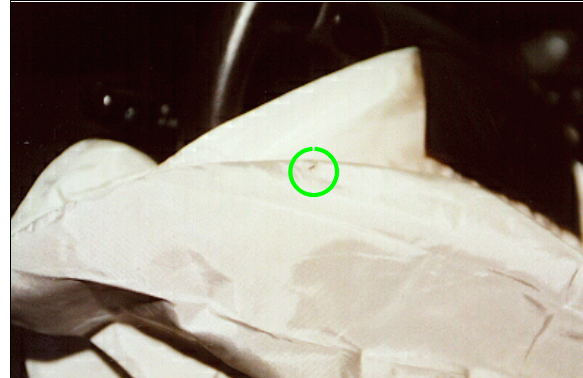
Figure 11: Close-up of cut/hole near seam in top portion of case vehicle's deployed driver air bag (case photo #33a)
