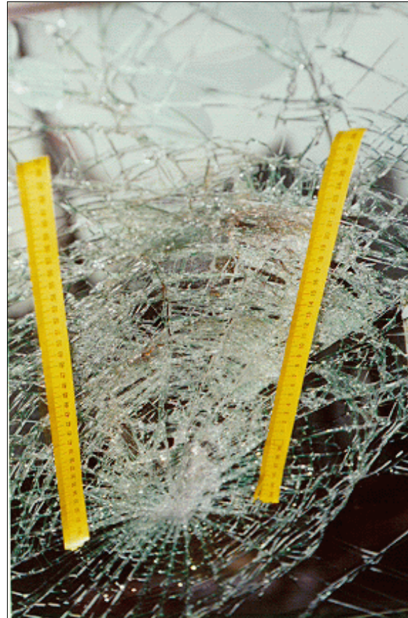
Figure 6: Close-up of large skin transfer to interior surface of case vehicle's right windshield glazing (case photo #36)
