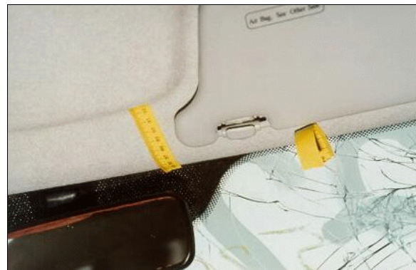
Figure 7: Close-up of contact scuff to case vehicle's front right header/sun visor; Note: rear view mirror tilted toward driver (case photo #38)
