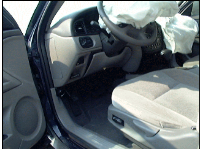
Figure 4. Driver's seated position—shows left knee contact
