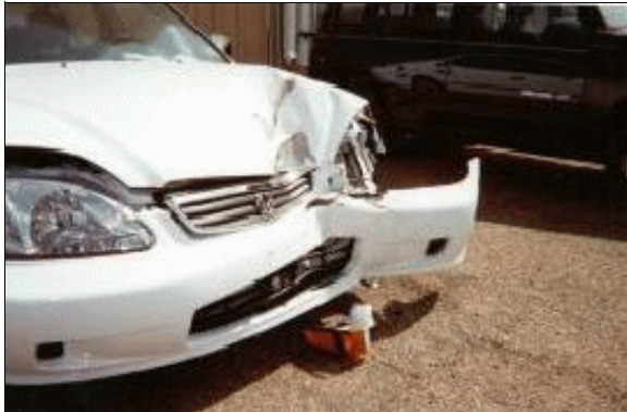
Figure 7: Case vehicle's front left half damage from utility pole impact viewed from right of front (case photo #05)
