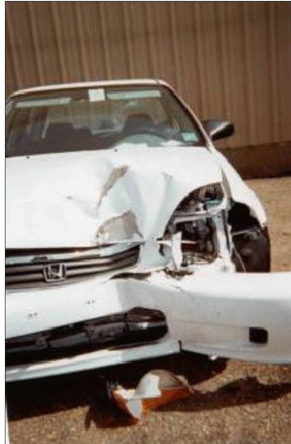
Figure 2: Case vehicle's front left half damage from utility pole impact (case photo #13)
