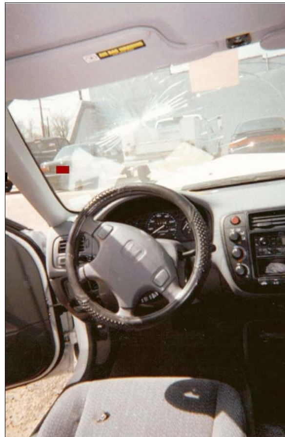
Figure 6: Vertical view of case vehicle's driver seating area showing unidentified object on driver's seat, non-deployed driver air bag, and crack to windshield (case photo #15)
