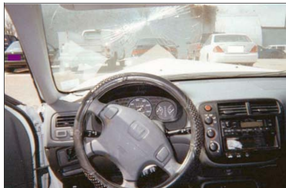
Figure 5: Case vehicle's driver seating area showing non-deployed driver air bag module and contact to windshield (case photo #14)
