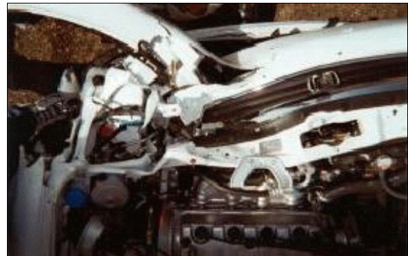
Figure 12: Overhead view of damage to case vehicle's front left half from impact with utility pole (case photo #12)
