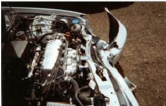
Figure 11: Case vehicle's damaged front left half viewed from right front with hood raised (case photo #09)
