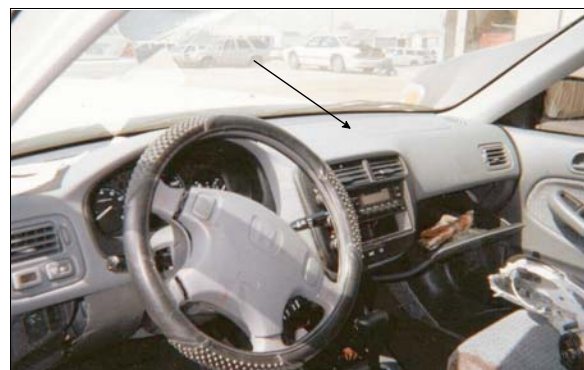
Figure 3: Case vehicle's front seating area showing non-deployed driver (steering wheel-mounted) and front right passenger (top instrument panel-mounted) air bags (case photo #02)
