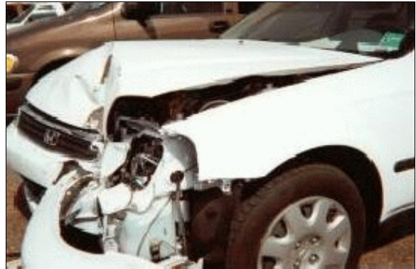
Figure 8: Case vehicle's frontal damage from utility pole impact viewed from left of front (case photo #03)
