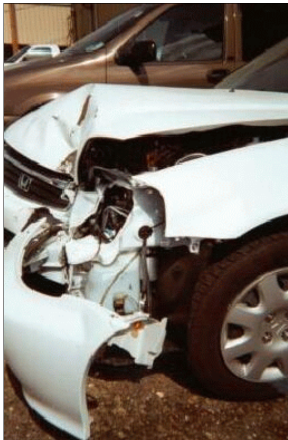
Figure 9: Closer-up vertical view of case vehicle's frontal damage from utility pole impact viewed from left of front (case photo #04)
