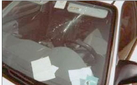
Figure 4: Close-up of crack to driver's side of case vehicle's windshield; Note: crack resulted from contact by case vehicle's driver (case photo #11)
