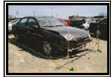
Figure 4. Frontal damage to the 1994 Geo Prizm.
