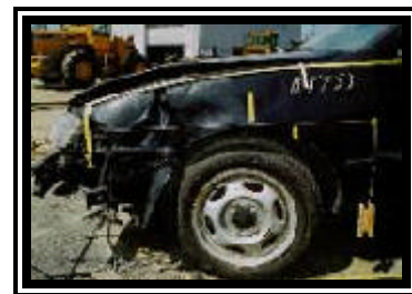
Figure 7. Opposing vehicle damage to the left front side surface.
