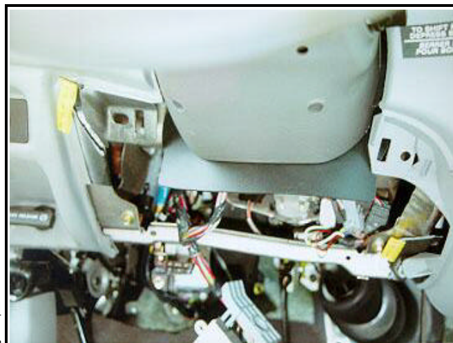
Figure 4. Deformed knee bolster.
