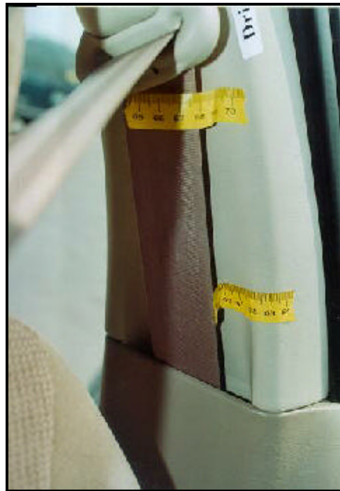
Figure 9. Load marks to driver's seat belt
