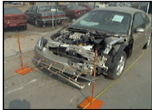
Figure 2. Exterior frontal damage to case vehicle.
