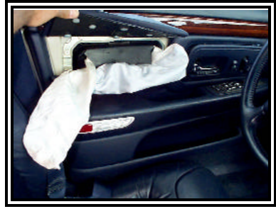
Figure 7. Air bag membrane and the module flap system.
