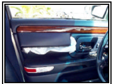
Figure 4. Left side impact air bag module.
