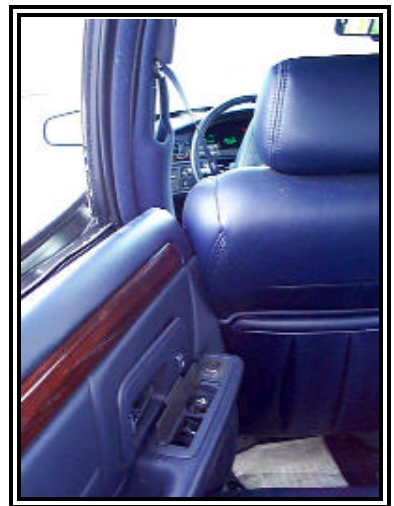
Figure 3. Intrusion of the left door and B-pillar components.
