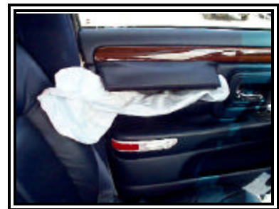
Figure 8. Expanding side impact air bag.
