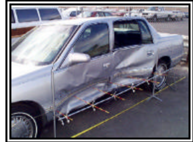
Figure 1. Left side damage to the Cadillac
