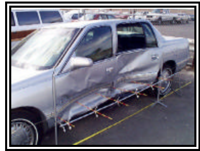
Figure 2. Left side damage to the Cadillac.
