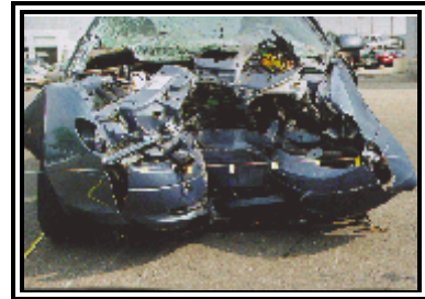
Figure 1. Frontal view of the impact damage to the 2000 Ford Taurus.
