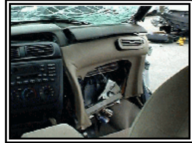
Figure 8. Non-deployment of front right air bag.
