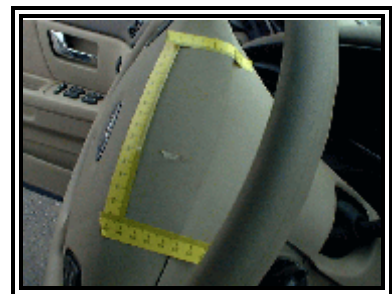
Figure 10. Driver contact evidence on steering wheel hub/air bag module cover.
