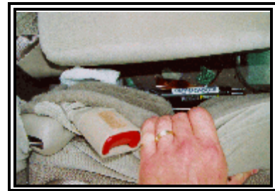
Figure 5. Passenger side fired pretensioner.
