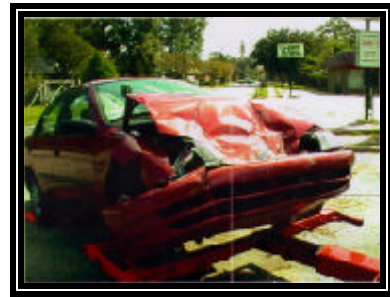
Figure 5. Frontal damage to the Chevrolet Metro
