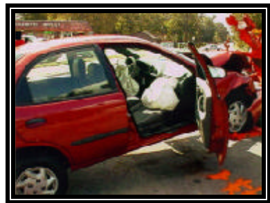
Figure 6. Right side view of the frontal damage
