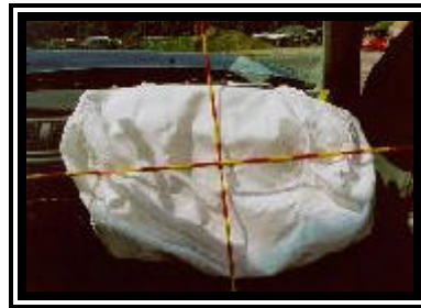
Figure 6. 2000 Ford Taurus LX deployed redesigned passenger air bag.
