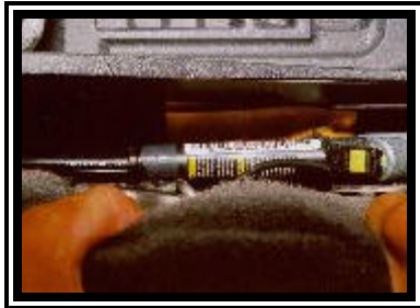
Figure 7. Front left restraint activated belt pretensioner.
