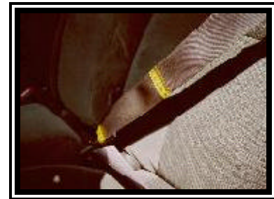
Figure 3. Loading marks to the front left shoulder belt webbing.
