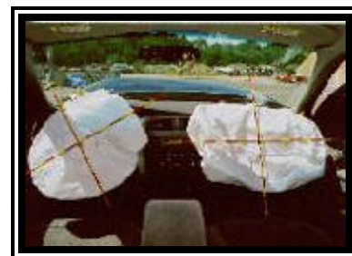
Figure 4. 2000 Ford Taurus LX deployed frontal air bags.
