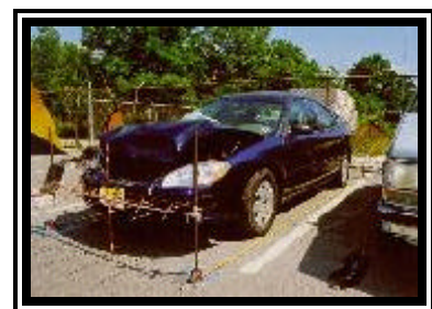
Figure 2. Frontal damage to the 2000 Ford Taurus LX.
