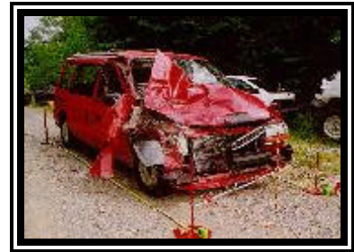
Figure 5. Frontal damage to the 1995 Plymouth Voyager.
