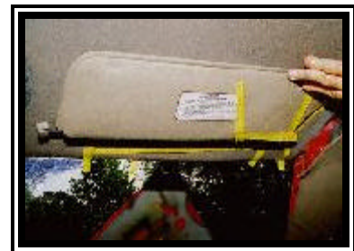
Figure 7. Contact evidence to the sunvisor and windshield header.
