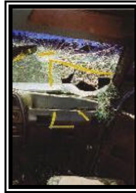
Figure 9. Contact evidence to the front right passenger space.
