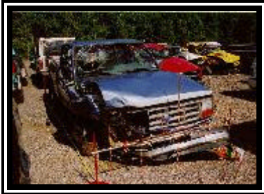
Figure 6. Frontal damage to the 1991 Ford Ranger XLT 4x4 pickup truck.
