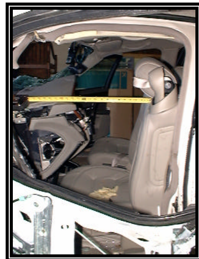
Figure 7. Forward deflection of seat back and rearward intrusion of the steering column and instrument panel.
