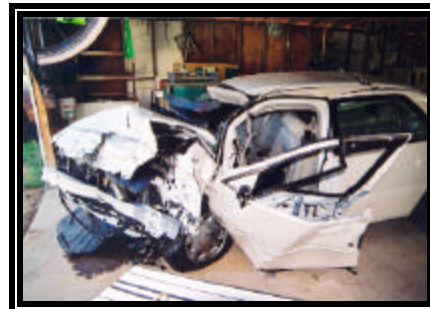
Figure 6. Lateral view documenting the extent of frontal crush.
