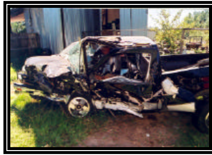
Figure 9. Continuous engagement onto the left side of the Nissan.
