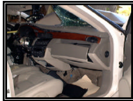
Figure 11. Non-deployed front right air bag.
