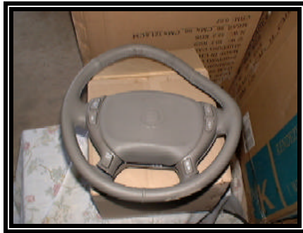
Figure 10. Separated steering wheel with non-deployed air bag module.
