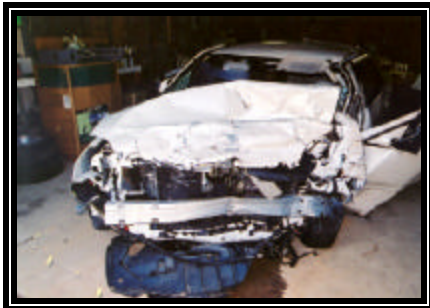
Figure 5. Frontal damage to the Cadillac DeVille.
