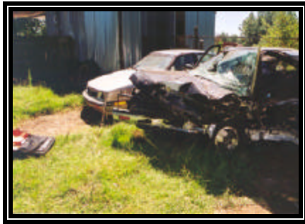
Figure 8. Extent of frontal crush to the Nissan KingCab.
