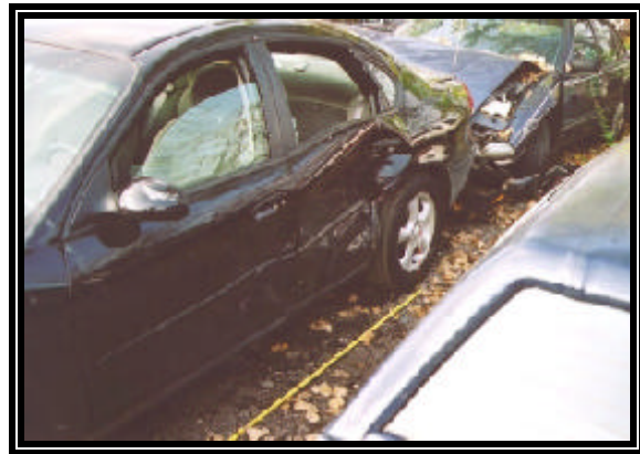
Figure 4: View of the side slap damage to the Taurus SE.
