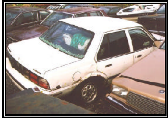
Figure 6: Right rear side slap damage.
