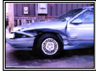
Figure 11. Side damage to the Ford Taurus
