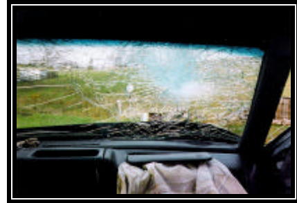
Figure 7. Interior view showing windshield damage
