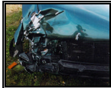
Figure 6. Frontal damage showing maximum crush
