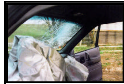
Figure 8. Frontal air bag system in the Voyager
