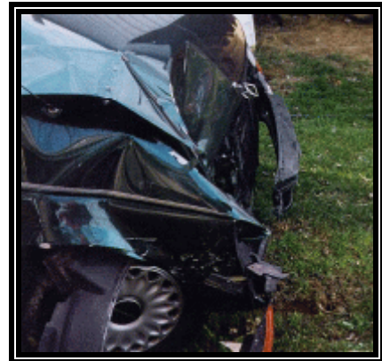
Figure 5. Lateral view of frontal damage
