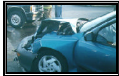
Figure 3. Damage to the left bumper corner and left fender
