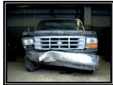
Figure 8. Frontal damage to Ford F-150 pickup truck
