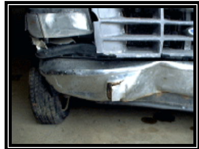
Figure 9. Displaced right frame rail protruding through bumper
