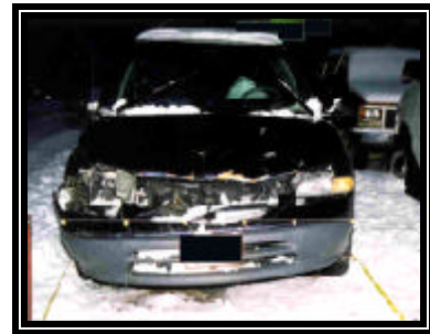
Figure 13. Frontal damage to 1997 Dodge Grand Caravan
