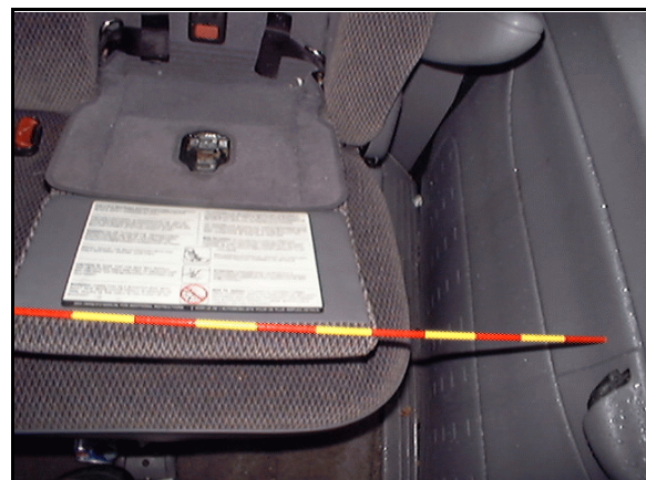
Figure 7: Second row left CSS cushion open on bench seat cushion, showing door panel intrusion
