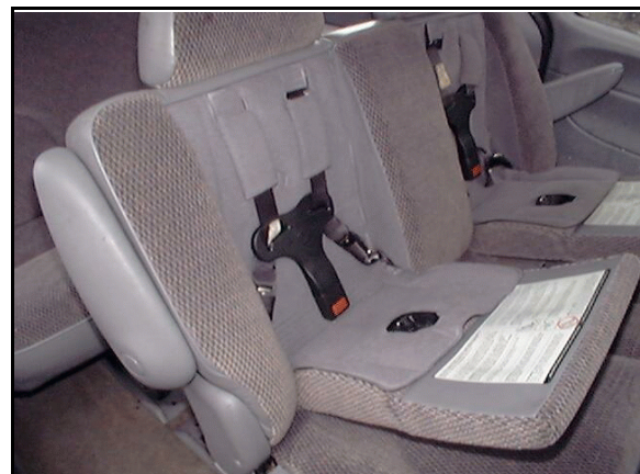
Figure 5: Case vehicle's second row bench seat with two integral child safety seats folded open
