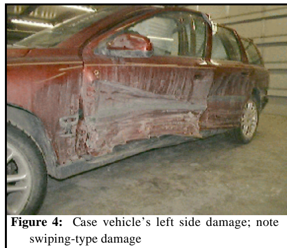
Figure 3: Case vehicle's left side damage
