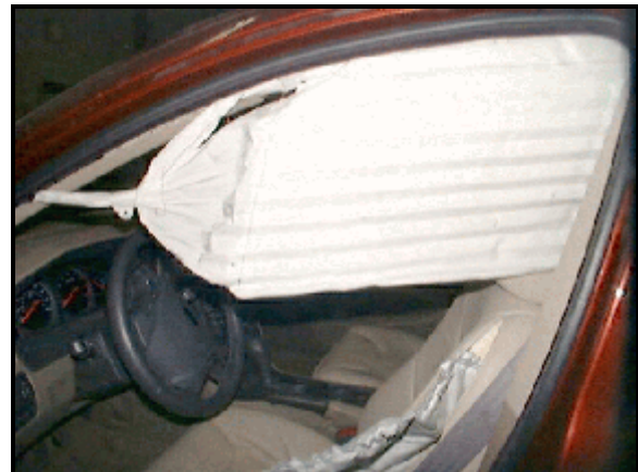
Figure 7: Left roof rail-mounted inflatable curtain, forward portion viewed from outside
