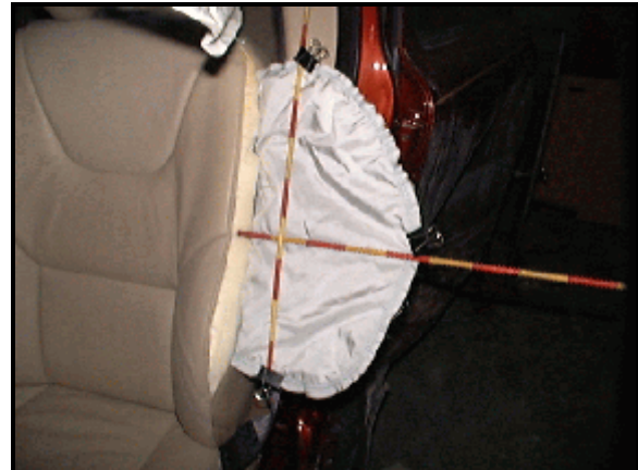
Figure 5: Deployed driver's seat back-mounted side air bag, showing inboard surface
