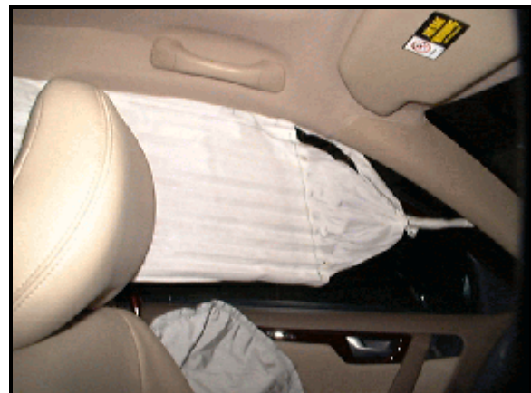
Figure 8: Interior view of left roof rail-mounted inflatable curtain, forward portion
