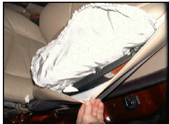
Figure 6: Deployed driver's seat-back mounted side air bag, showing module and outboard surface
