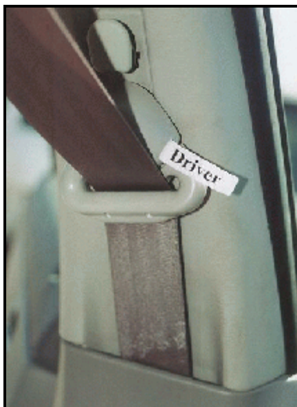
Figure 9. Load marks to driver's seat belt
