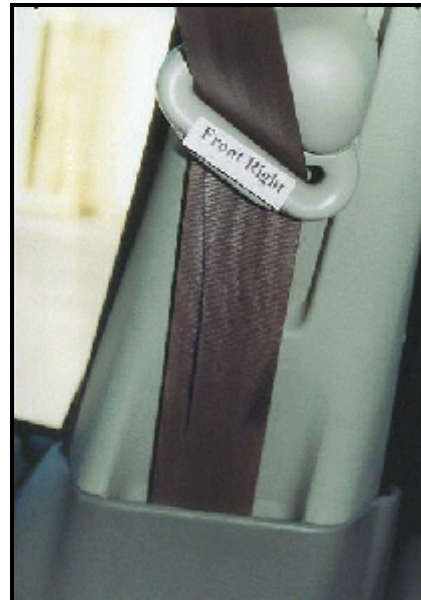
Figure 10. Load marks to front right passenger seat belt
