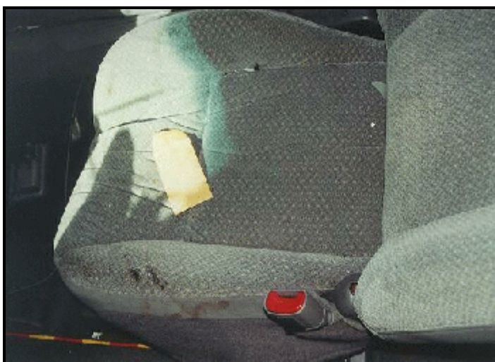
Figure 11. Ride-down pattern in front right seat
