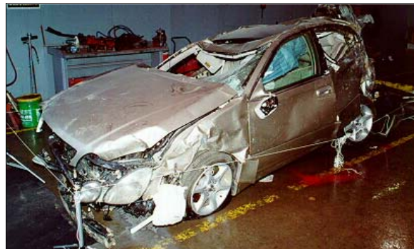
Figure 17: Deformation to case vehicle from frontal and multiple rollover impacts viewed from front portion of left side (case photo #05)
