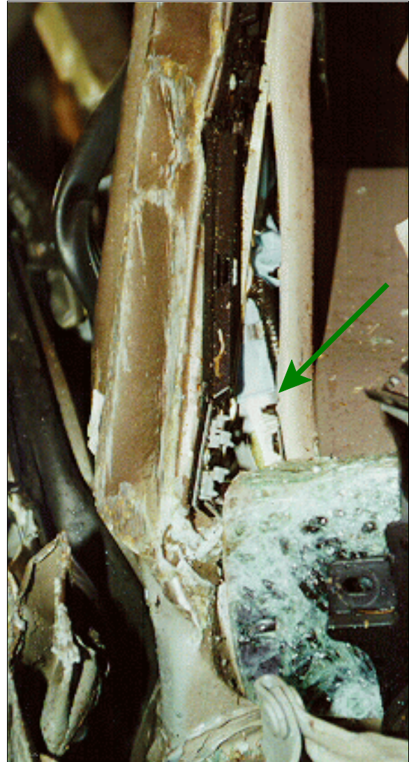
Figure 33: Close-up of exposed exhaust cannister stored in base of right "A"-pillar for case vehicle's non-deployed, right side inflatable curtain (case photo #52)
