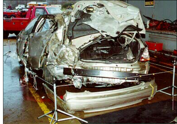
Figure 10: Deformation to case vehicle's back left corner viewed from left of back; Note: mud and grass stuck in left "C"-pillar (case photo #09)
