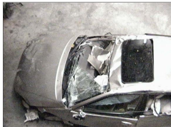
Figure 15: Overhead view of deformation to case vehicle's front; Note: rightward shift of hood in response to impact with 1 st culvert's embankment (case photo #107)
