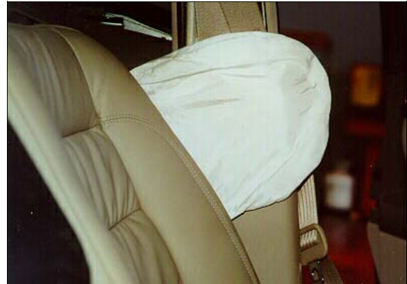
Figure 24: Close-up of interior portion of case vehicle's deployed, driver seat back-mounted, side air bag showing no visible contact evidence (case photo #39)
