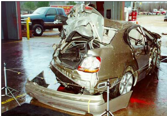
Figure 11: Deformation to case vehicle's back viewed from right of back; Note: damage occurred during vehicle's end-over-end rollover impact with 2 nd culvert's embankment (case photo #14)
