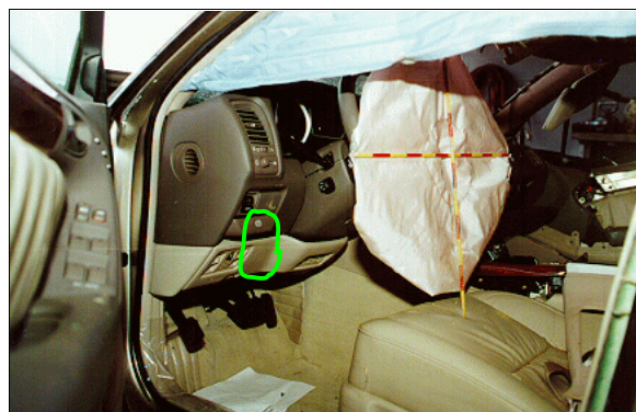
Figure 18: Case vehicle's driver seating area showing driver's deployed front air bag and side inflatable curtain; Note: minimal floor pan intrusion and left knee contact to driver's knee bolster (case photo #28)
