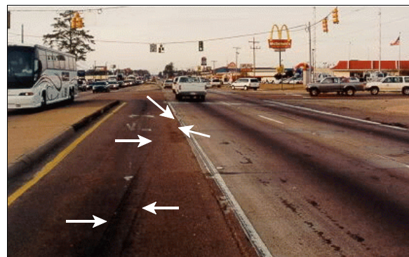
Figure 2: On-site view showing sharply turning critical curve scuff deposited in left-hand turn lane as case vehicle's driver swerved rightward into through lanes and began traveling northbound across roadway (case photo #67)
