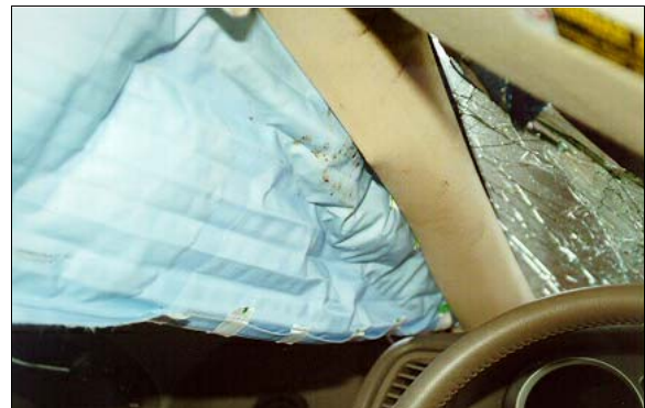
Figure 26: Close-up of front interior portion of case vehicle's deployed driver side inflatable curtain showing blood evidence (case photo #32)
