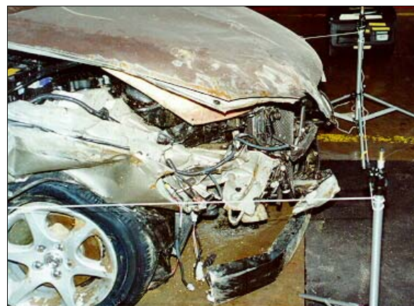
Figure 8: Reference line view from right of deformation to case vehicle's front right corner as a result of impact with 1 st culvert's embankment (case photo #22)
