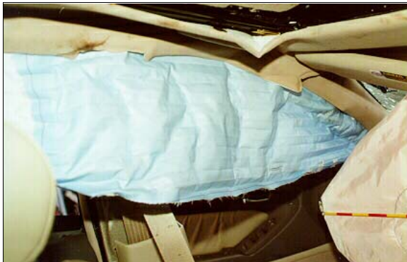
Figure 25: Case vehicle's deployed driver side inflatable curtain viewed from back right seat; Note: collapsed roof and left "A"-pillar (case photo #31)
