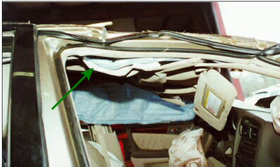
Figure 34: Case vehicle's exposed, non-deployed, right side inflatable curtain which was stored between right side rail and roof (case photo #54)
