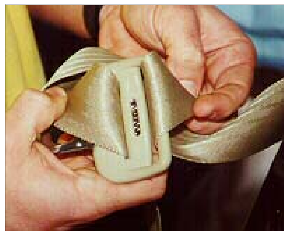
Figure 28: Close-up of heavy friction mark on plastic latch of case vehicle's driver seat belt (case photo #44)
