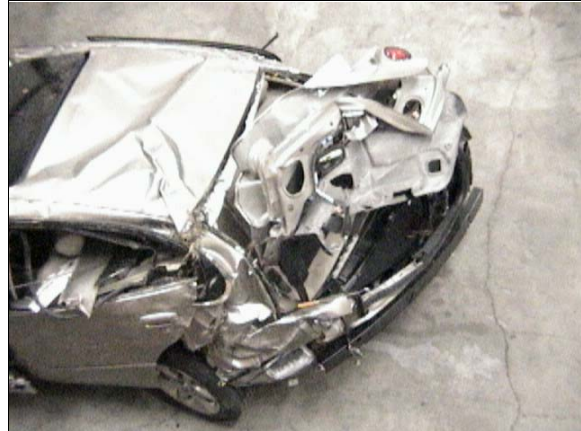
Figure 16: Overhead view of deformation to case vehicle's back showing non-horizontal impact direction to back left corner from impact with 2 nd culvert's embankment (case photo #108)
