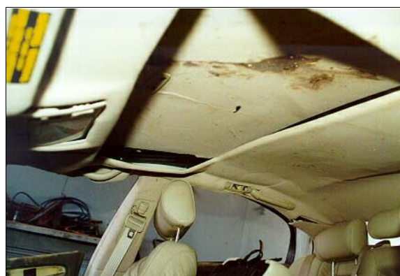
Figure 31: Case vehicle's roof viewed from driver's seating position showing numerous marks and blood stains; Note: adjustable head restraints and front upper anchorages (case photo #64)
