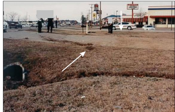
Figure 12: On-scene view of area where case vehicle landed after rolling over (i.e., rotation about both longitudinal and lateral axes) following its impact with the 2 nd culvert's embankment (closest arrow); case vehicle continued to roll about its longitudinal axis, coming to rest on the north side (farthest arrow) of the 3 rd driveway (case photo #86)
