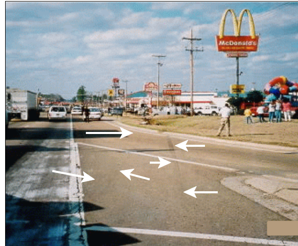
Figure 3: On-scene view of case vehicle's northward travel path from inside through lane onto eastern shoulder prior to departing road; Note: tire yaw marks leading off road toward curb indicate driver's attempt to steer leftward back toward roadway (case photo #69)
