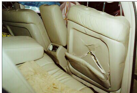
Figure 20: Damage to back surface of case vehicle's front right seat back from loading by back right passenger (case photo #58)
