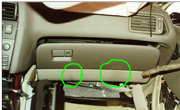
Figure 19: Contact evidence (highlighted) on case vehicle's front right knee bolster, just below glove box door from front right passenger's knees (case photo #46)
