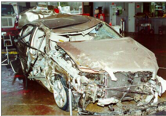
Figure 7: Deformation to case vehicle's front from impacts with sign, 1 st culvert's embankment, and subsequent rollover impacts, viewed from right of front (case photo #23)
