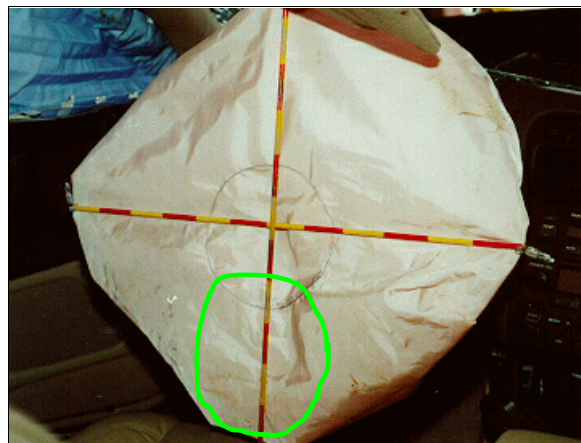
Figure 22: Case vehicle's deployed driver air bag showing area (highlighted) of bloody and oily smears (case photo #33)
