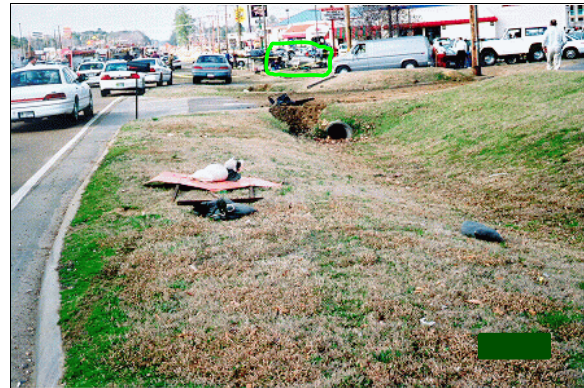
Figure 5: On-scene view looking in a northerly direction at case vehicle's path of travel through warning sign (2 nd impact) and into culvert's embankment (3 rd impact); Note: ground dugout during embankment impact and final rest position (highlighted) of case vehicle (case photo #74)
