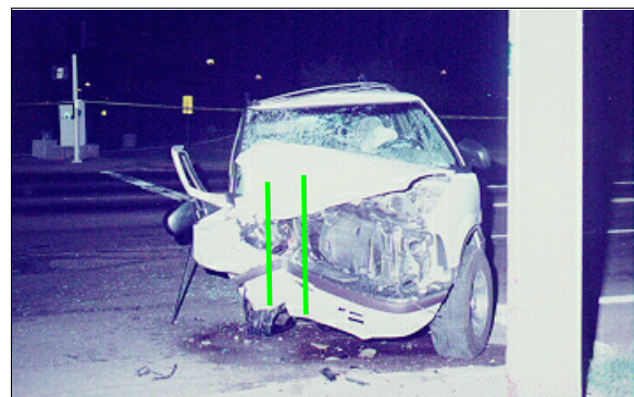
Figure 5: On-scene view looking north-northeast at case vehicle's final rest position; Note: pole impact (highlighted) location (case photo #14)
