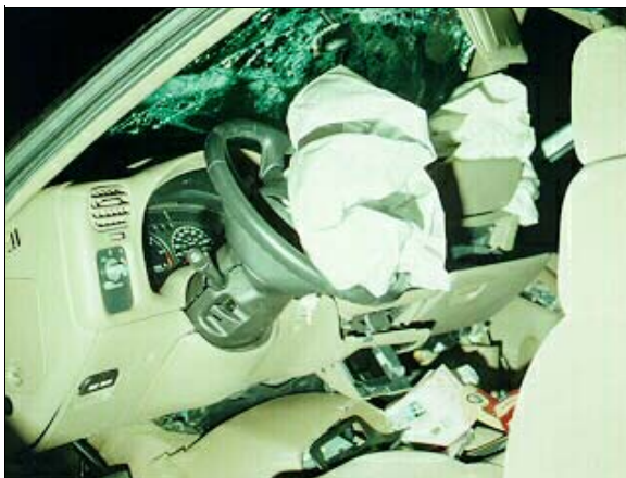
Figure 11: On-scene view of case vehicle's driver seating area showing deployed air bags and intrusion to right instrument panel (case photo #17)
