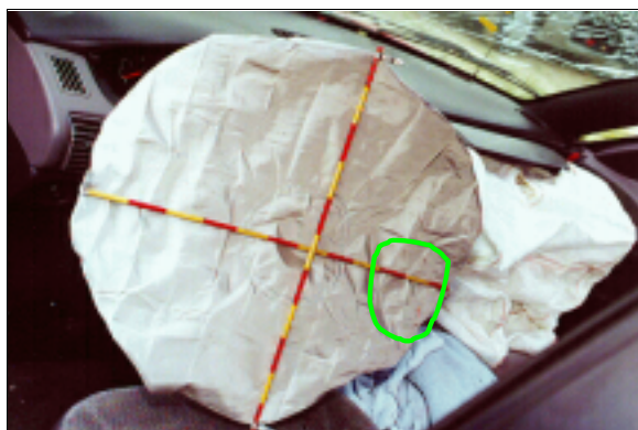
Figure 14: Case vehicle's driver air bag showing area of contact evidence (skin, mascara, and blood) highlighted (case photo #29)
