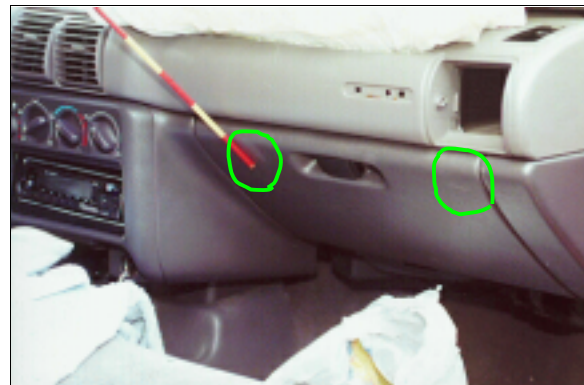
Figure 13: Contacts to case vehicle's glove box by front right passenger's thighs (case photo #35)
