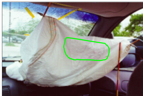
Figure 16: Case vehicle's deployed front right passenger air bag showing more pink cloth transfers on bottom surface (case photo #37a)
