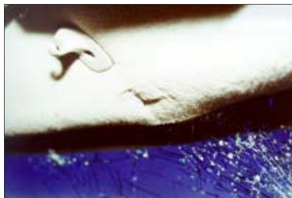
Figure 21: On-scene close-up of evidence (i.e., hair and indentation) on case vehicle’s right windshield header from contact by front right passenger (case photo #68)
