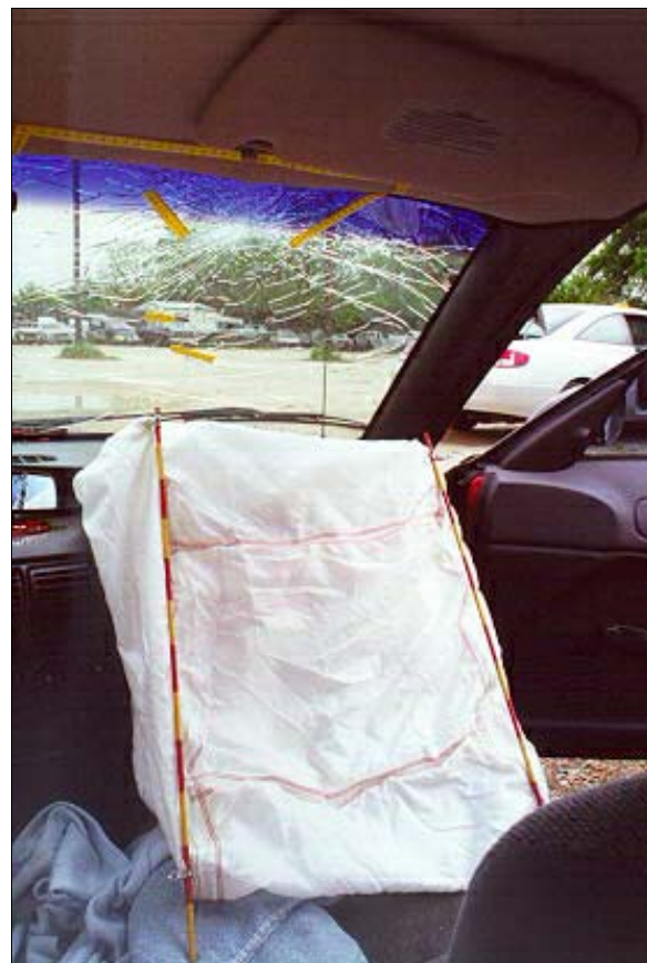
Figure 10: Vertical view of case vehicle's deployed front right passenger air bag; Note: pink cloth transfer to air bag's front surface and contacts to windshield's glazing and header, and sun visor (case photo #37)
