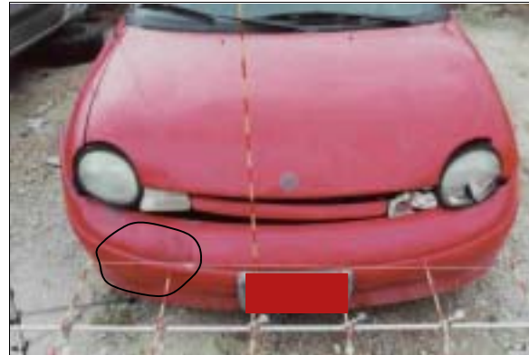
Figure 8: Elevated view of case vehicle's frontal damage with contour gauge present on bumper; Note: black scuffs toward front right corner are from Chevrolet's left rear tire (case photo #12)
