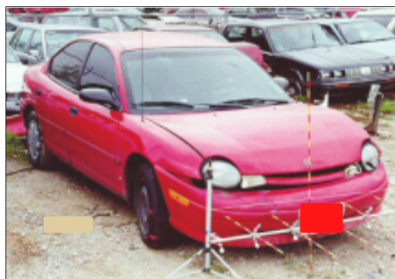
Figure 3: Case vehicle's damaged front with contour gauge present (case photo #24)
