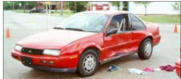
Figure 5: On-scene view of Chevrolet's left side damage; Note: Chevrolet is heading southwest (case photo #70)
