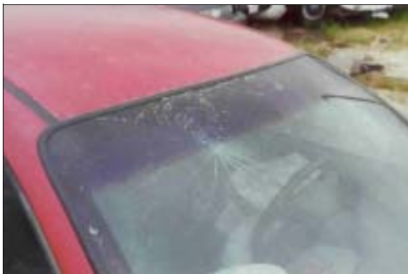
Figure 9: Exterior view of impacts to case vehicle's right front windshield glazing (case photo #25)
