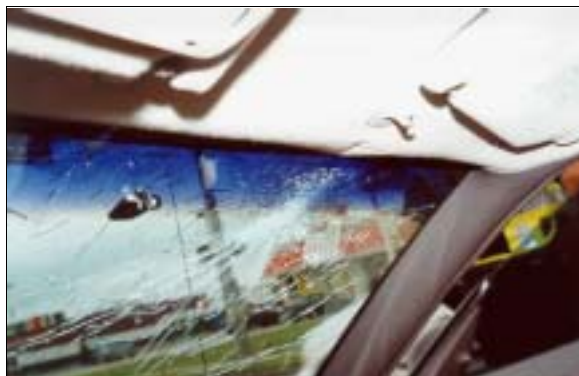
Figure 20: On-scene view from driver’s seat showing dislodged rear view mirror and contacts to right windshield’s glazing and header (case photo #69)
