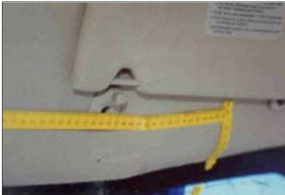
Figure 12: Case vehicle's contacted front right windshield header toward left side of front right sun visor showing hair and indentation in header (case photo #38)
