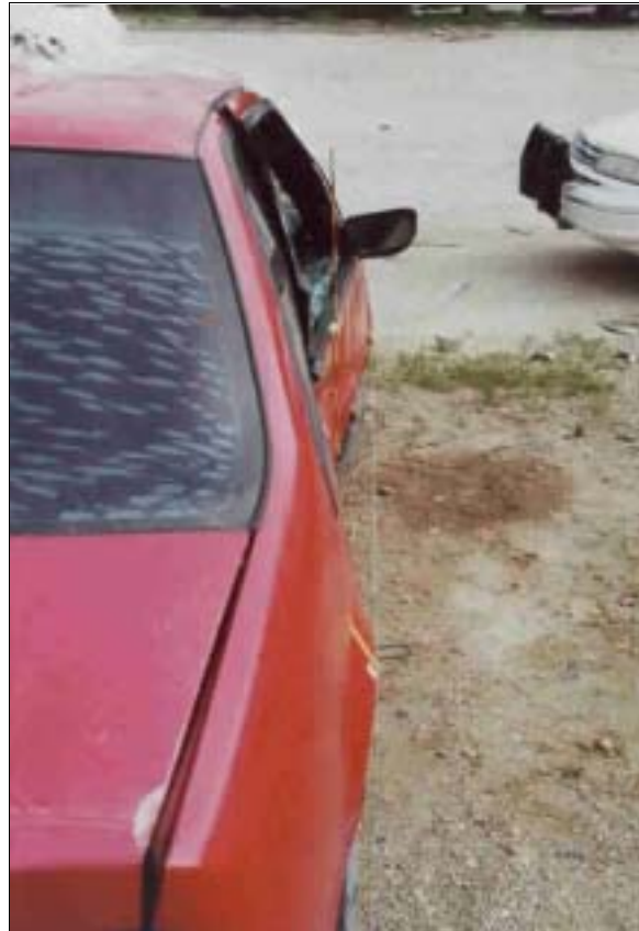
Figure 26: Chevrolet's left side damage viewed from front along stringline (case photo #62)
