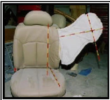
Figure 9. 2000 Infinity I30 deployed left front side impact air bag.
