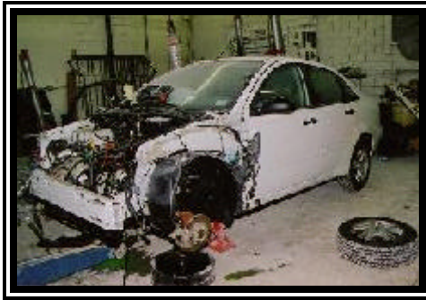
Figure 5. Frontal damage to the 2000 Ford Focus SE 4-door sedan.
