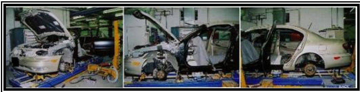
Figure 3. Left side surface damage to the 2000 Infinity I30 4-door sedan.
