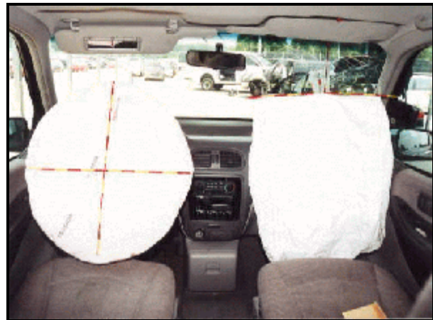
Figure 4. Full frontal view of case vehicle interior showing deployed air bags
