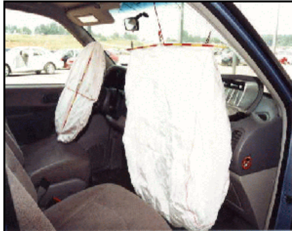
Figure 6. Front, right view showing deployed frontal air bags.
