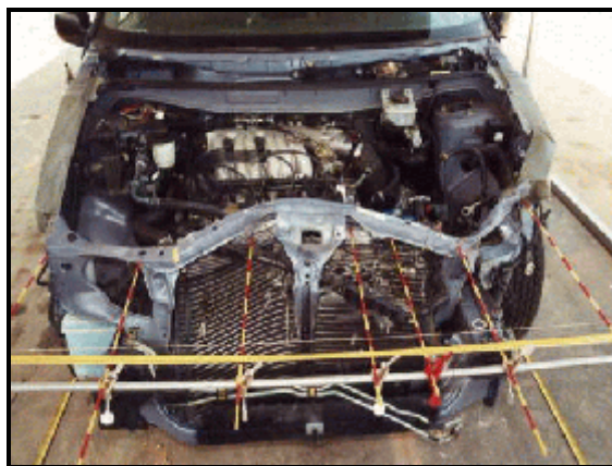
Figure 2. Frontal overhead view showing frontal deformation to case vehicle
