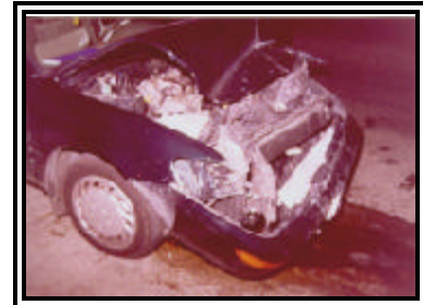
Figure 1. Frontal damage to the 1996 Toyota Corolla
