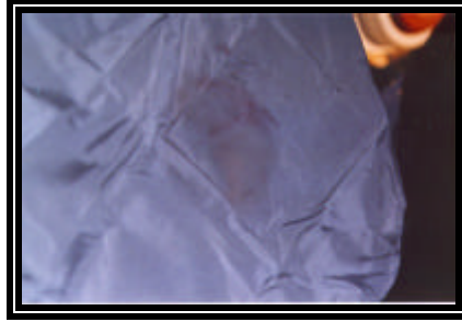
Figure 6. Probable makeup transfer on driver's air bag
