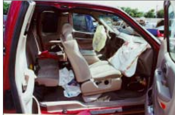
Figure 6: Case vehicle's interior with both right side doors open showing super cab and deployed front air bags (case photo #28)
