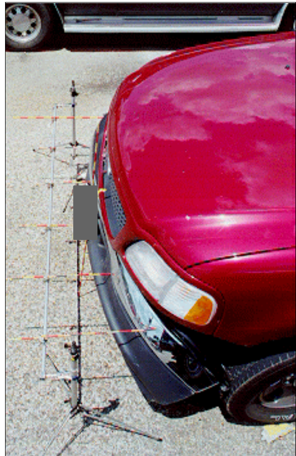
Figure 8: Reference line view of minor deformation to case vehicle's front bumper (case photo #09)
