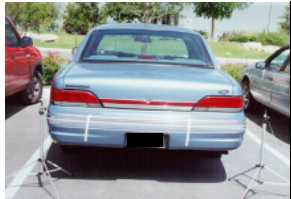
Figure 3: Ford Crown Victoria's impacted back bumper showing outline (between tape) of direct damage (case photo #31)
