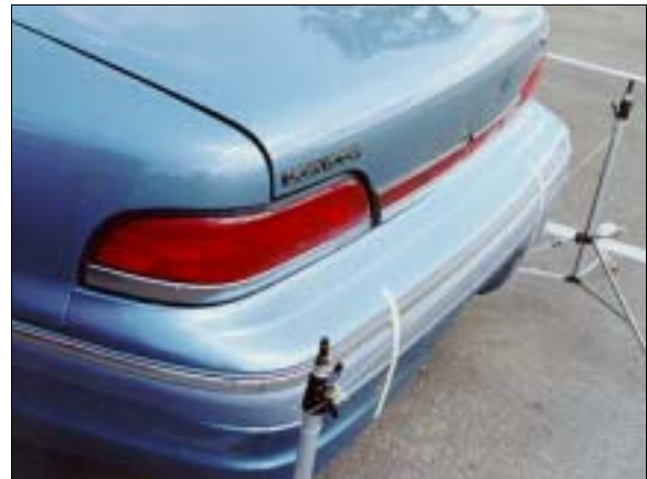
Figure 20: Ford Crown Victoria's back showing width of direct contact on bumper and slight separation of trunk lid as only visible deformation (case photo #46)
