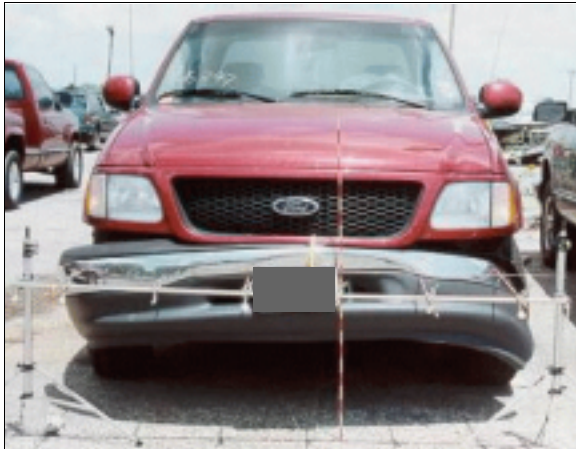
Figure 2: Case vehicle's frontal damage with contour gauge present; Note: bumper rotated upward (case photo #08)
