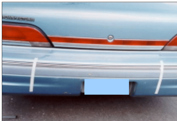
Figure 21: Ford Crown Victoria's back bumper damage with tape indicating length of direct contact; Note: only very minor damage was found (case photo #47)
