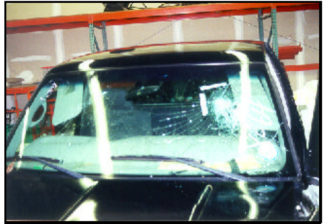
Figure 9. Exterior view of windshield contact
