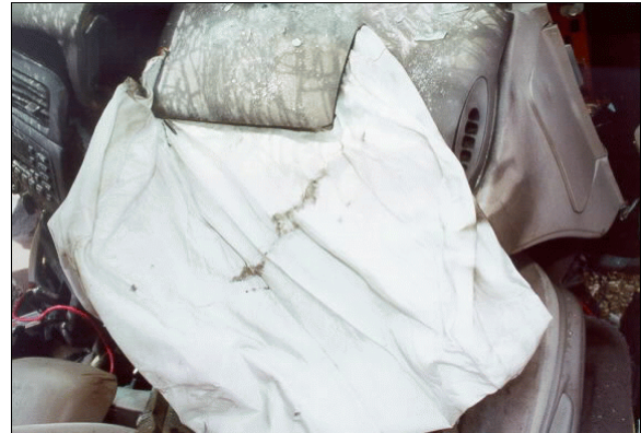
Figure 12: Case vehicle's front right module cover flap and deployed air bag showing snagging and tears to top surface (case photo #55)
