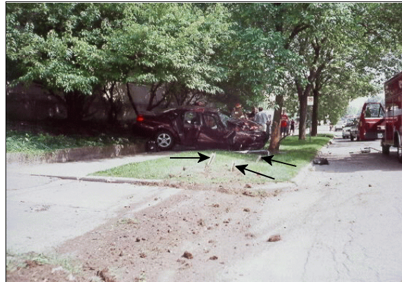
Figure 3: On-scene, case vehicle's path, showing soil thrown by undercarriage impact, sign posts (arrows), and final rest (case photo #72)
