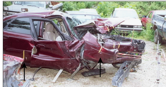
Figure 6: Case vehicle's right side showing front deformation, right front wheel off, and side swipe damage (tape) (case photo #25)
