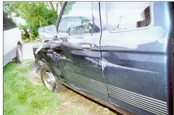
Figure 13: Sideswipe damage to Ford Ranger pickup's left side (case photo #65)
