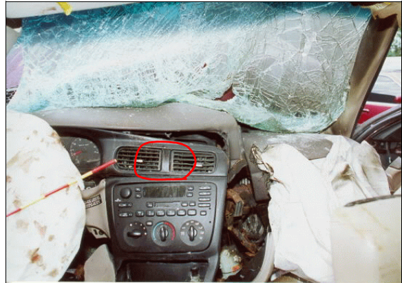
Figure 10: Case vehicle's center and front right area showing intrusion, driver contact evidence on center instrument panel, cracked and holed windshield glazing, deployed front right air bag, and fire damage to right instrument panel area and below (case photo #46)
