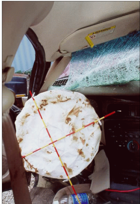
Figure 11: Case vehicle's driver seating area showing driver's deployed bloodstained air bag, cracked windshield glazing, and blood evidence on driver's sun visor (case photo #40)
