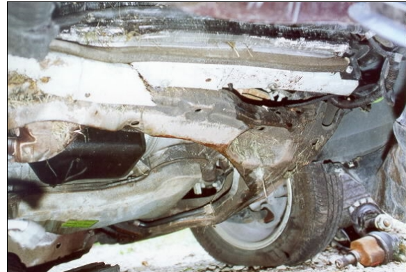
Figure 8: Undercarriage view from front of direct contact to case vehicle's front frame members with embedded grass (case photo #30)
