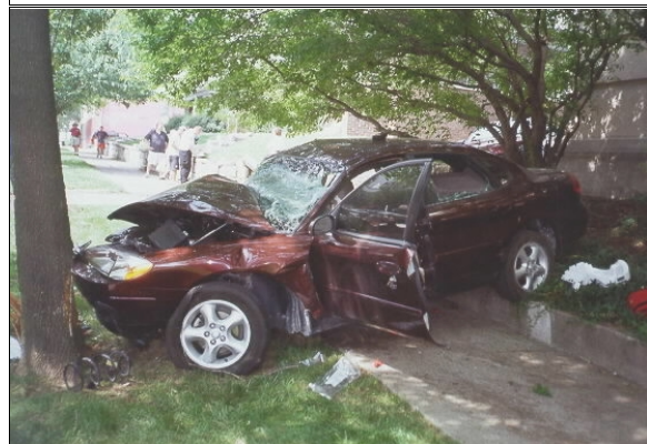
Figure 5: On-scene view of case vehicle's final rest position, straddling sidewalk with rear tires up over concrete knee wall (case photo #75)
