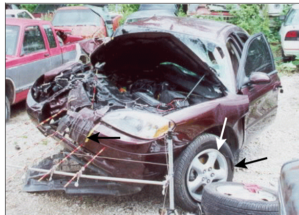
Figure 7: Front left view of case vehicle's damage; Note: tape on bumper (arrow) indicates 2nd sign post impact; damaged left front wheel/tire; right front wheel/tire broken off (case photo #17)
