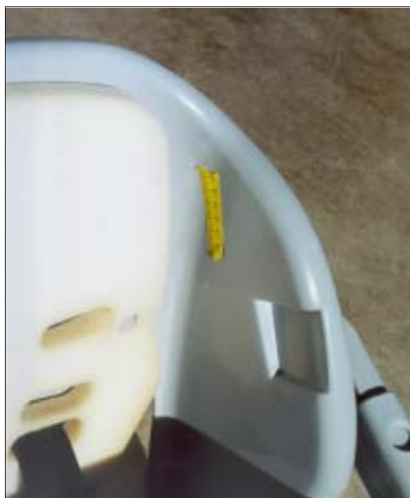
Figure 19: Close-up of child safety seat used by case vehicle's back center passenger showing small stress area to upper left corner of plastic shell (case photo #58)
