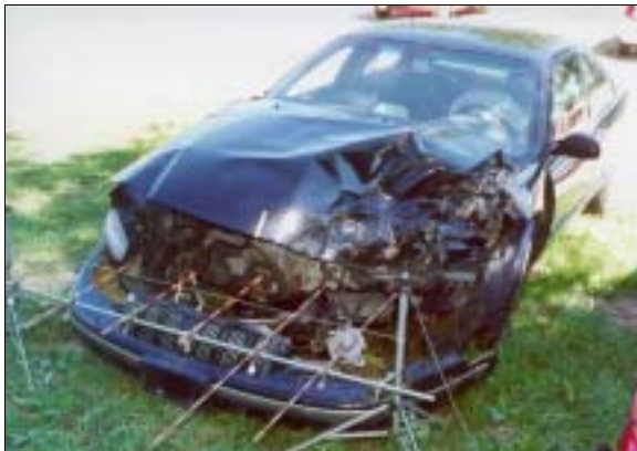
Figure 3: Elevated view from left of front of case vehicle's frontal deformation with contour gauge present showing damage from impact with Pontiac and traffic signal pole (case photo #18)
