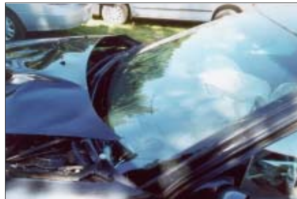
Figure 12: Stress fracture to case vehicle's windshield caused by back left tip of hood (case photo #24)
