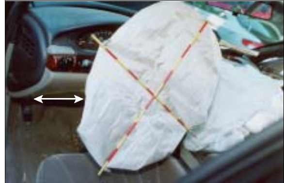
Figure 15: Case vehicle's deployed driver air bag showing small red transfer in center of air bag's stitching and contact (i.e., tape) to knee bolster (case photo #45)
