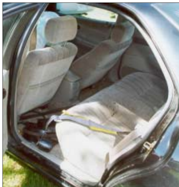
Figure 21: Case vehicle's back seat showing loading evidence (yellow taped area) to center lap belt (case photo #51)
