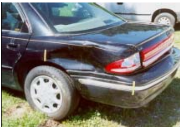
Figure 5: Case vehicle damaged left quarter panel from side slap impact with Pontiac; Note: yellow tape marks direct contact width (case photo #25)
