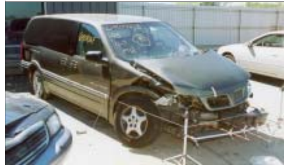
Figure 4: Pontiac's front right deformation viewed from right of front with contour gauge present showing impact from case vehicle; Note: side slap damage to right rear (case photo #73)
