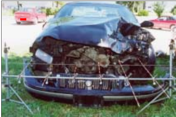
Figure 10: Case vehicle's overlapping frontal damage from four frontal impacts—Pontiac, Chevrolet, traffic signal pole, and wood pile (case photo #17)
