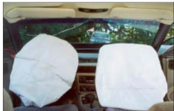
Figure 17: Case vehicle's deployed front air bags; Note: absence of contact evidence to windshield's glazing and sun visors (case photo #44)
