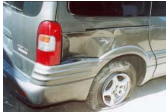
Figure 24: Pontiac's right back damage viewed from right of back, resulting from side slap impact with case vehicle's left back (case photo #70)
