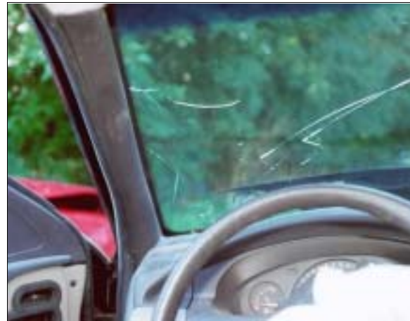
Figure 13: Case vehicle's left "A"-pillar and windshield's glazing showing scratches on "A"-pillar from rings on driver's left hand and stress fracture of windshield's glazing (case photo #38)
