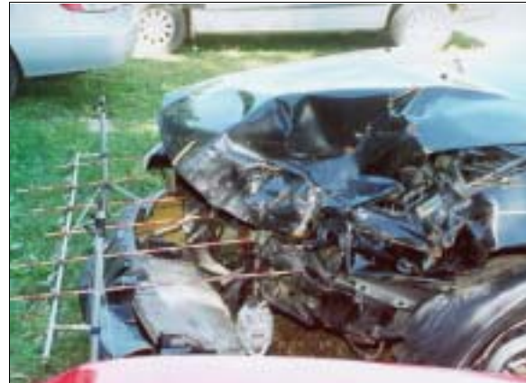
Figure 11: Reference line view from left showing case vehicle's damage from Pontiac and traffic signal pole (case photo #21)
