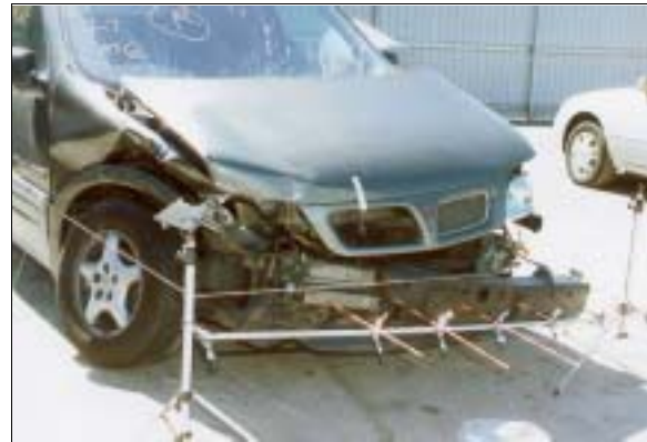
Figure 23: Pontiac's front right damage viewed from right of front from impact with case vehicle; Note: left shifted front bumper and yellow tape marks width of direct contact (case photo #74)
