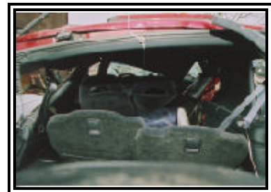
Figure 9. View from backlight of interior damage to the Chevrolet Blazer
