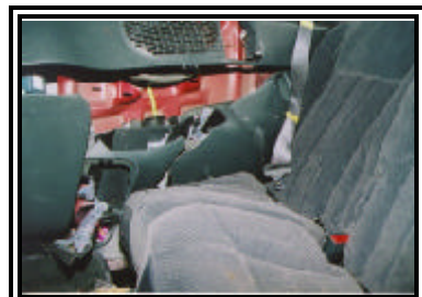
Figure 16. Scuff marks on interior trim panel from shield booster seat
