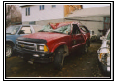
Figure 7. Trip-over damage to the Chevrolet Blazer
