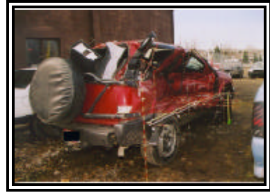
Figure 6. Right side damage to Chevrolet Blazer
