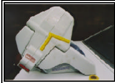
Figure 15. Scuff marks on shield booster seat
