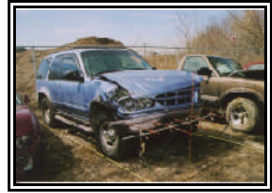
Figure 11. Frontal damage to the Ford Explorer
