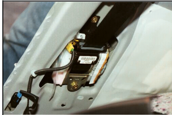
Figure 7: Front right passenger's safety belt retractor-type pretensioner (case photo #39)
