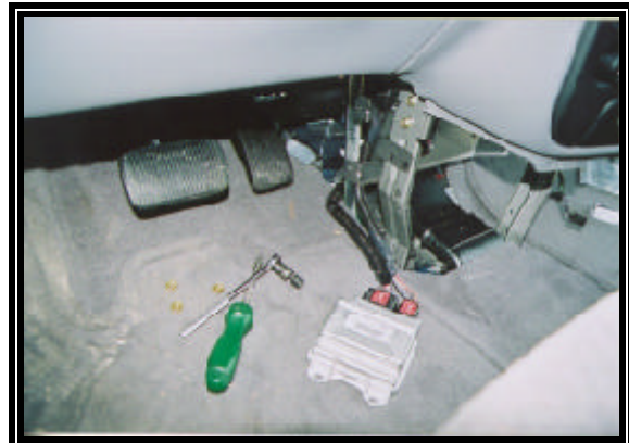
Figure 6: View of the Restraint Control Module during removal.
